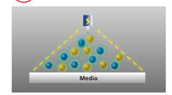
Static electricity on print media is one of the major factors that cause printing defects. The built-in on-carriage ionizer neutralizes static electricity and eliminates static related print issues, even in a low humidity environment.
