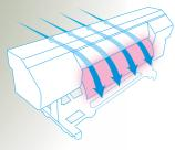
The air flow inside the printer has been redesigned for faster ink drying. The air flow system brings air from the rear of the printer and then blows it along the front cover out of the printer. This air flow coupled with a large heater makes it possible to quickly dry even low odor inks.
