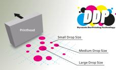
Dynamic Dot Printing Technology controls and optimizes dot size to produce rich, bold and glossy colors with fine details. DDP also creates high density printing without any loss in speed, giving the ColorPainter M-64s backlit film capabilities.
